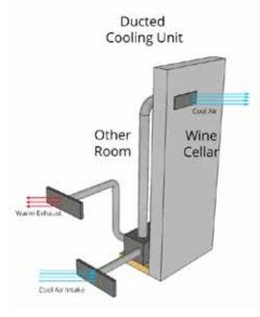
**Fully Ducted Cooling Unit** - a fully ducted cooling unit allows you to mount the cooling unit itself remotely (in a ceiling or utility room) and the use ducting to both blow the cool air in and exhaust the warm air.
